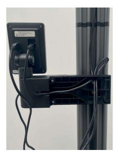
Plug the USB connector of the RFID reader on the back of the display into the free USB port and run the cable as depicted by the opening provided for this purpose.
