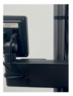
4. Carefully place the cover back on the display holder and run the excess cable in the guide of the aluminum profile. Finally, place the plastic cover on the aluminum profile to cover the cables.
