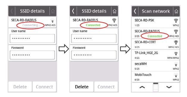
The seca mBCA 555 / seca TRU now establishes a connection to the selected WiFi network. As soon as the connection is established, it will be indicated by the message "Connected" behind the selected network.
